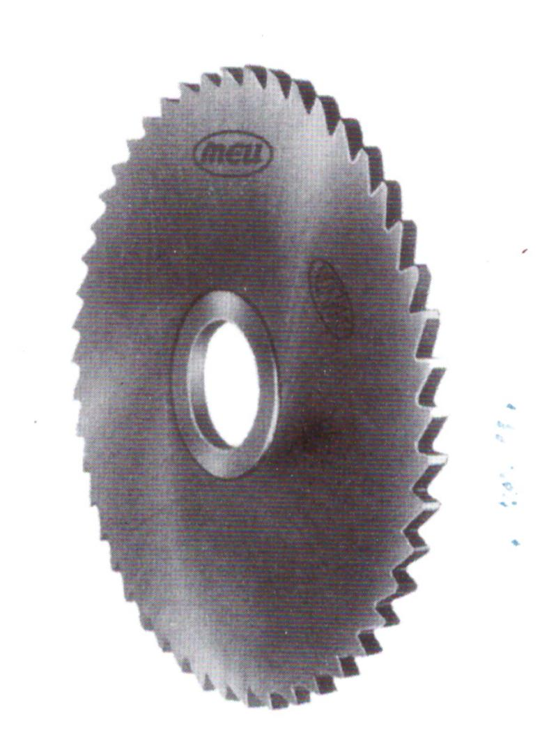
A cutter with teeth on the periphery only, not exceeding 6mm width and having side clearance.
