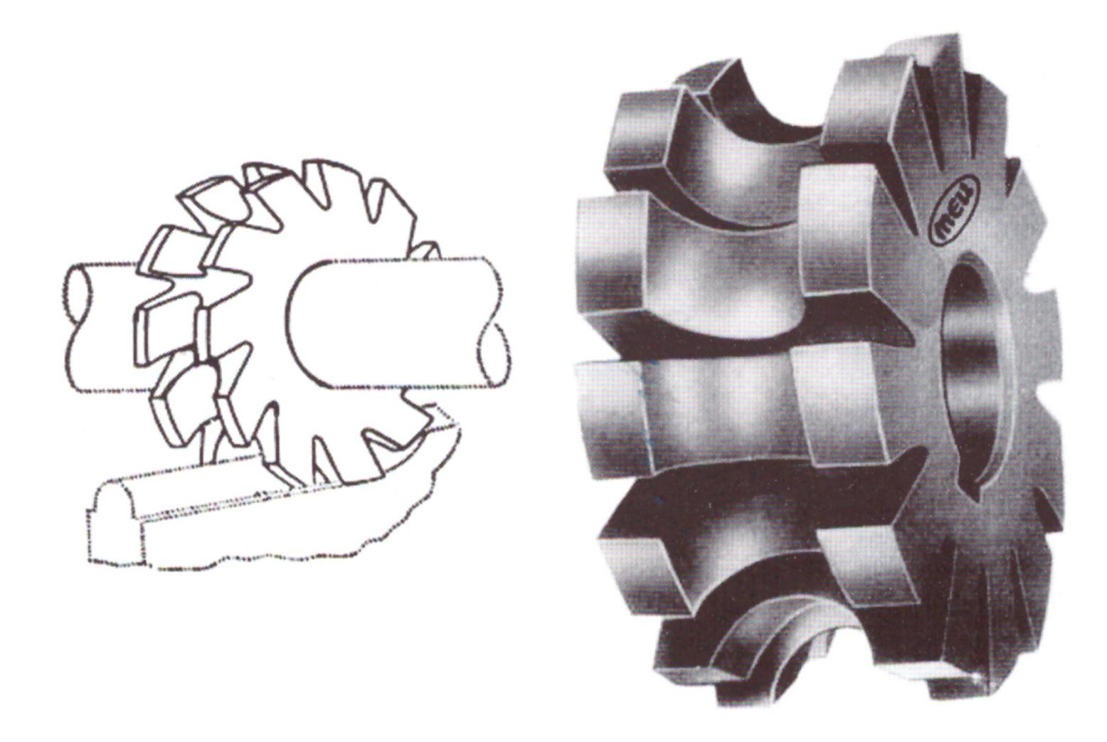
A cutter having a con-cave half circle in the form and having radially machine relieved teeth and tool Type 'N'.
