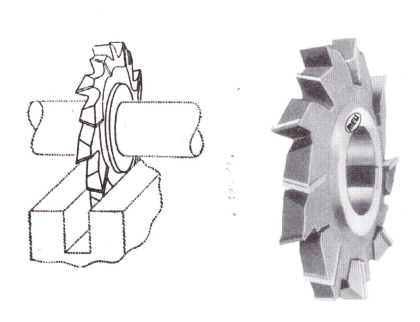
A Cutter with teeth on the periphery and on both sides. The teeth are alternately right-hand and left-hand angled and have a positive rake. Alternate side teeth are removed.
