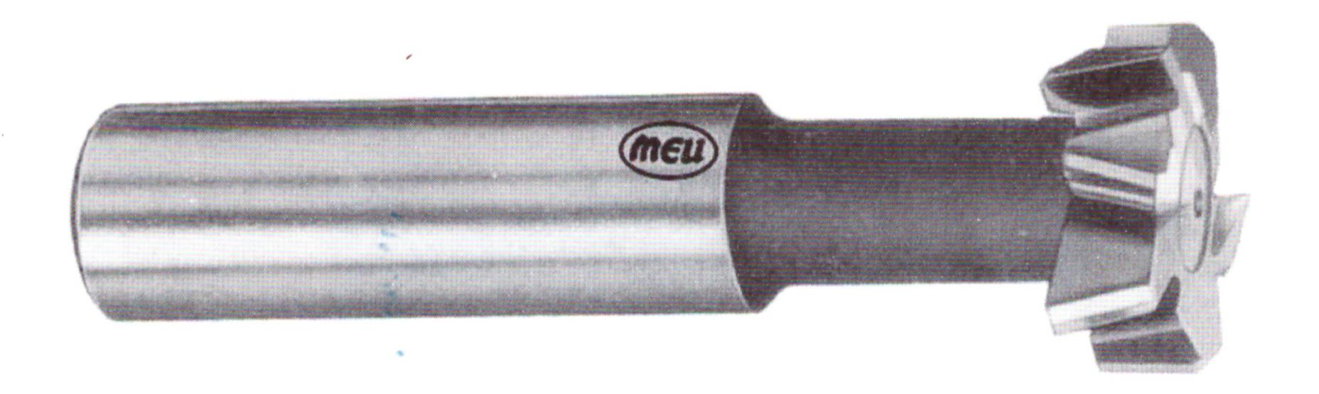
A cutter having the characteristics of a side and face cutter, integral with a parallel shank for holding and driving, and designed for cutting 'T' slots.
