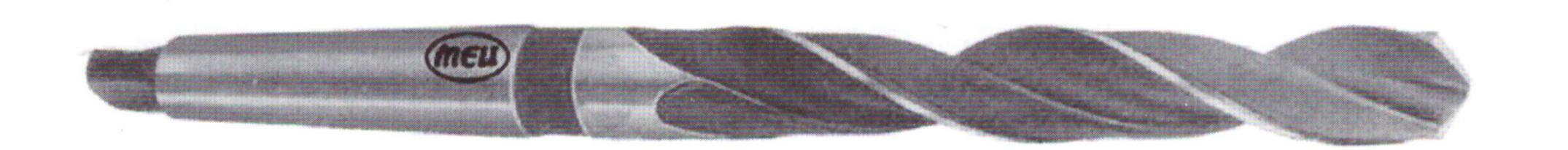
A drill having two helical flutes with a Standard Morse Taper Shank for holding and driving similar to a Standard Taper Shank Twist Drill, but with increased flute length.
